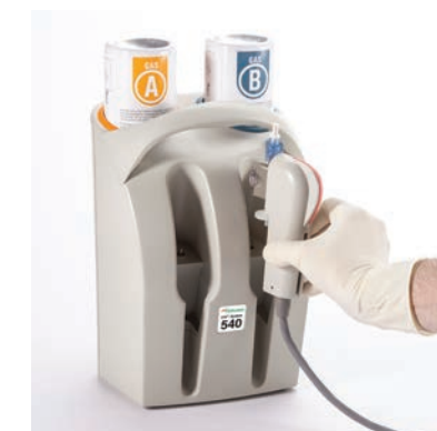
The cable head, with sensor attached, is placed in the calibrator.
